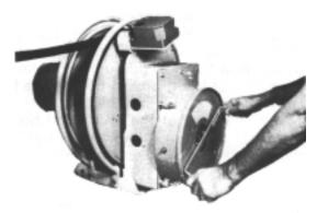
**Spring Tension Adjustment** — Spring tension can be increased from the outside by merely removing three screws and adjusting spring to tension as shown on nameplate. No need to disconnect cable or disassemble reel.
